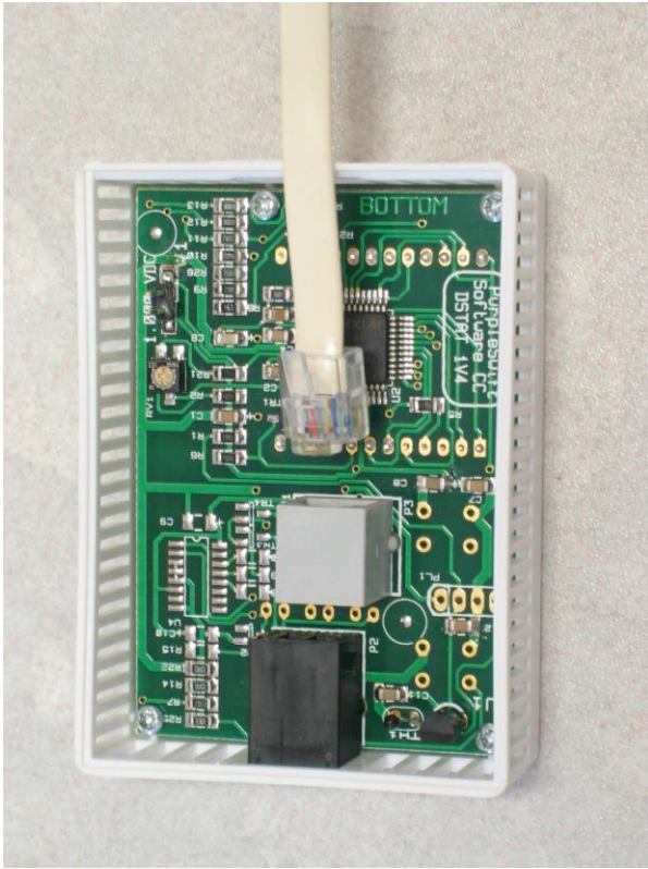
RMSTAT to D-Series controller RJ12 connection.
