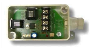
The D-SLAVE is a combination heater current valve and connection box designed for use with the D-Series DV1 VAV controllers.
