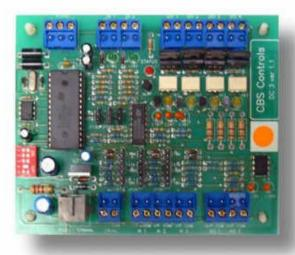
The **DC3** is a very cost effective extension of the Siemens Building Technologies System 600 BMS. It acts as a remote extension of the MBC or RBC. The system 600 programmer has access to the 11 points on the DC3. Each point can be unbundled and used in the usual manner including trending etc.
