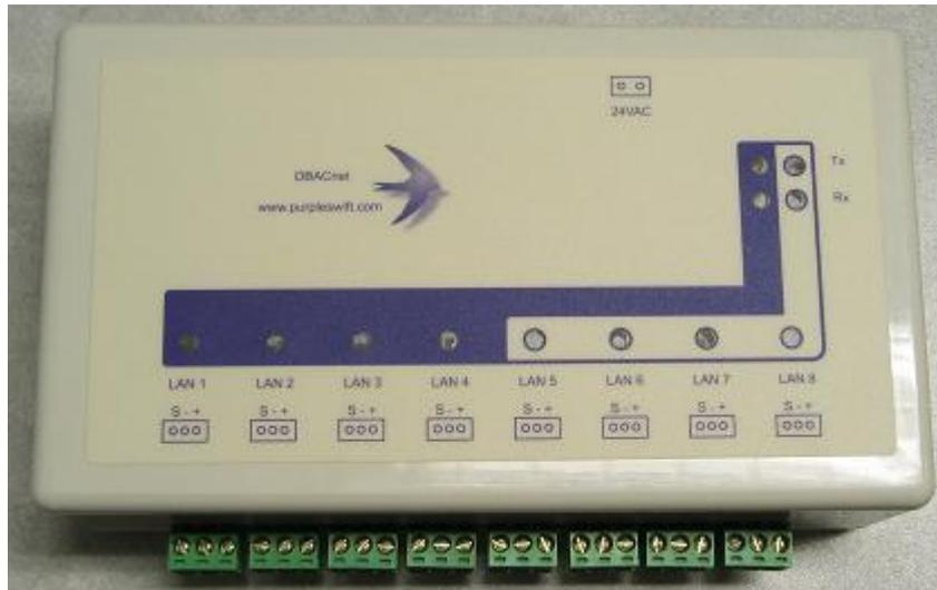
The DBACnet controller makes Siemens APOGEE floor level controls available to BACnet via the BACnet /IP protocol. The DBACnet controller communicates with any attached APOGEE floor level controls (such as the TEC) and makes the controls available to any BACnet system. The BACnet system can both read and write (command) the APOGEE device settings (sub-points).
